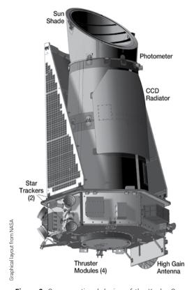
**Figure 2.** Cross-sectional design of the Kepler Space Telescope photometer instrument. Kepler is equipped with a 0.95 m (37 in) aperture Schmidt-type telescope and a 1.4 m (55 in) primary mirror. Kepler does not take photos but looks for dips in the light curve of a star that indicates a planet could be passing in front of it (called a transit).
